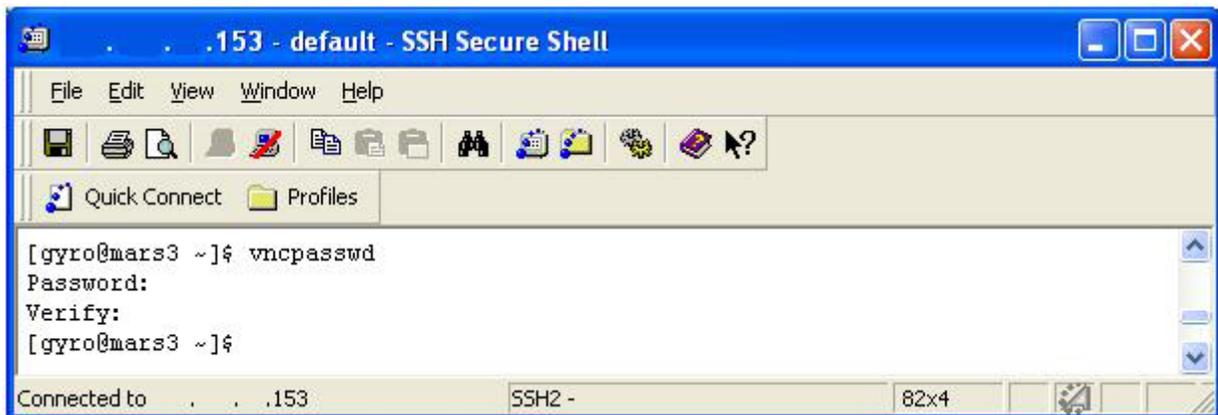
*Figure 1: Example of vncpasswd command*
