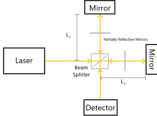
Figure 3: Shows the layout of a typical Michaelson Interferometer.
