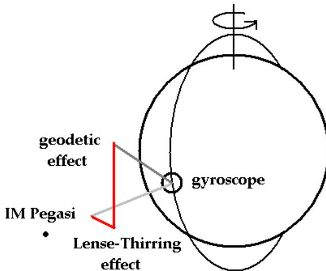
Figure 2: The precession of the spin of a gyroscope due to both Lense-Thirring and geodetic precession [2].
