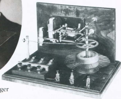
The original Strowger switch, for which he was granted a patent in 1891.
