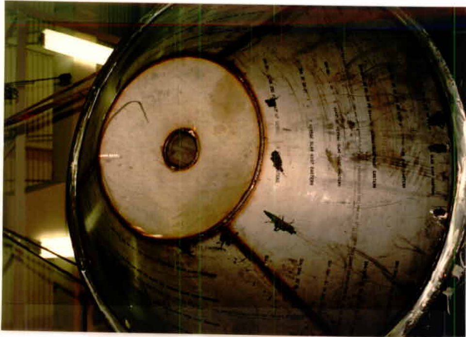
Fig. VII.1: Two views of one of the conical end tank segments (1 and 5). The outer shell of either of these two tanks carries 8 photomultiplier ports. Some of the stainless-steel flanges of the tank are visible in the upper portion of the figure.
