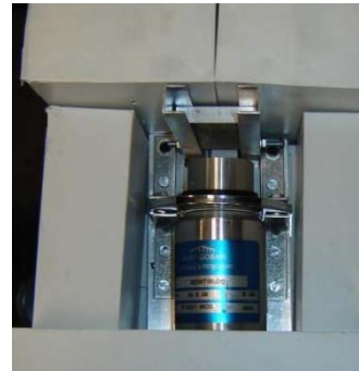
Low-level counting station with NaI counter (shielding partially removed).
