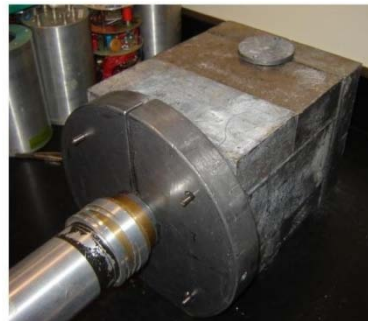
Low-level counting station with NaI counter (shielding partially removed).
