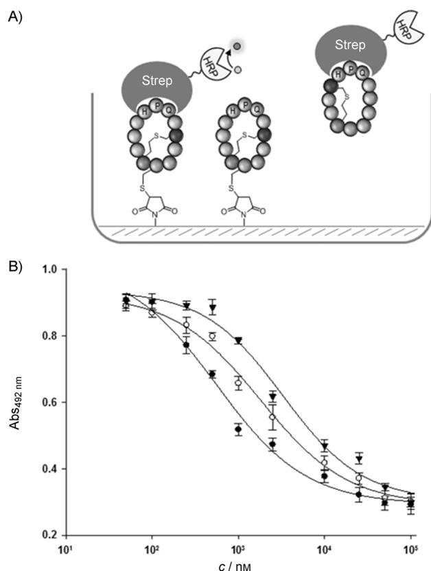
**Figure 2.** Streptavidin binding assay. A) Schematic representation of the inhibition assay. B) Inhibition curves for monocyclic peptide cyclo-Z3C (○;  $IC_{50} = (1.9 \pm 0.2) \mu\text{M}$ ) and bicyclic peptides bicyclo-Z3C (▼;  $IC_{50} = (3.7 \pm 0.2) \mu\text{M}$ ) and bicyclo-Z8C (●;  $IC_{50} = (0.77 \pm 0.08) \mu\text{M}$ ).
