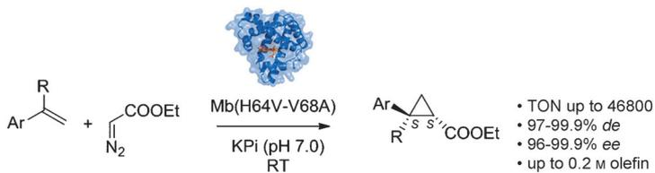
**The mediator:** A rationally designed myoglobin (Mb) catalyst capable of promoting the cyclopropanation of a range of aryl-substituted olefins with high catalytic activity and excellent diastereo- and
