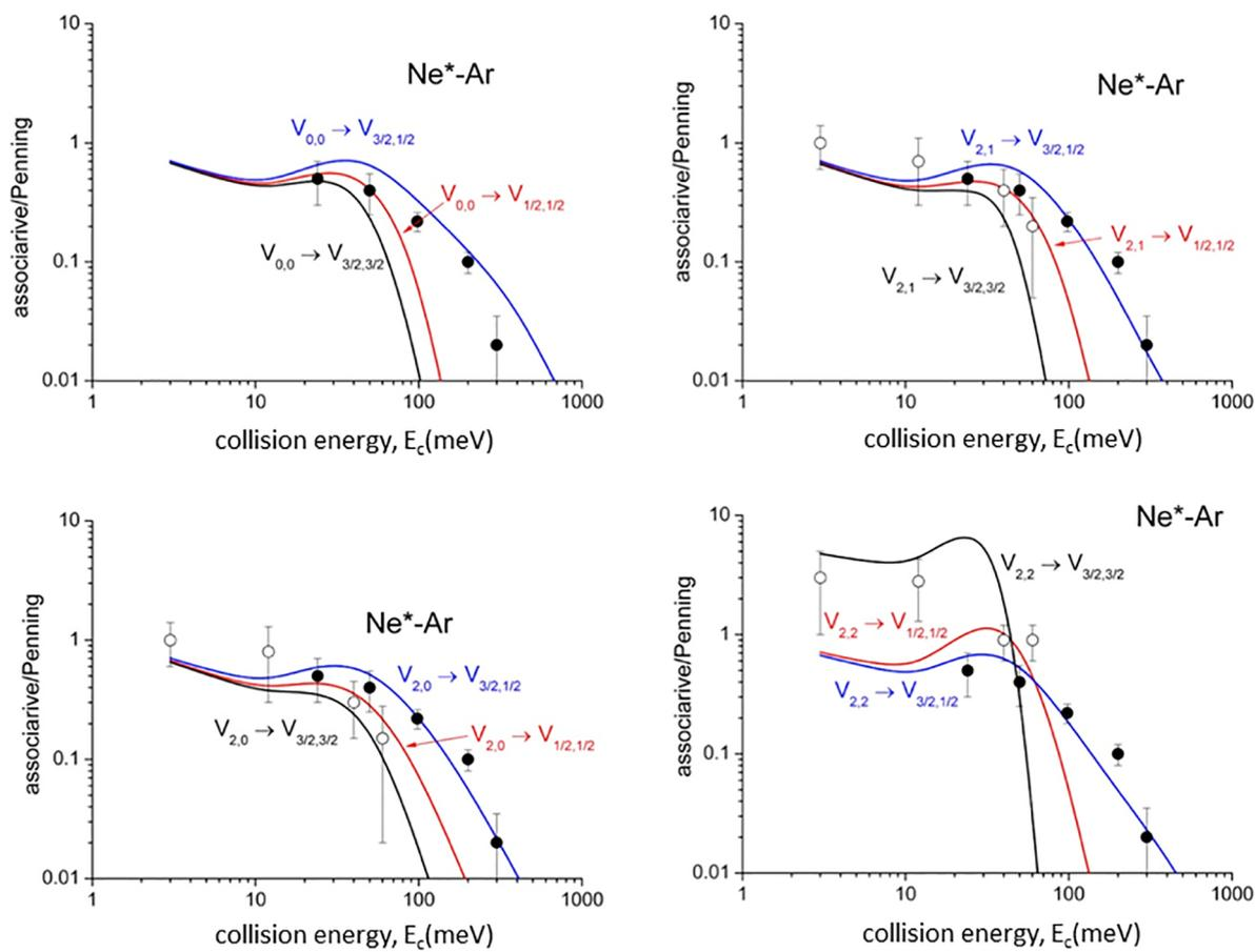
**Figure 6.** State-to-state associative/Penning ratios predicted for Ne\*–Ar. The comparison involves experimental results (black points, data from ref 51) referred to state averaged conditions. Recent data, measured with Ne\*( $^3P_2$ ) beams state-selected in  $\Omega = 2, 1, 0$  quantum states, are also reported (open circles) for a further comparison (data from refs 43–45).
