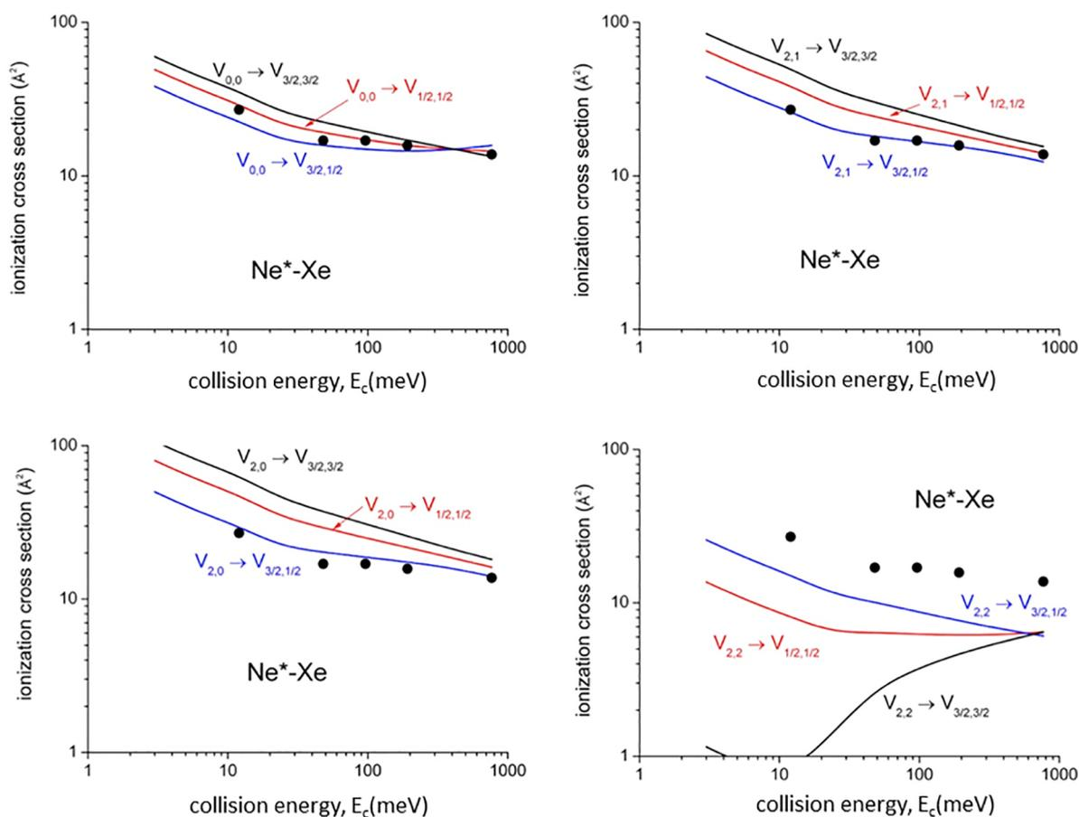
**Figure 5.** State-to-state total ionization cross section for  $\text{Ne}^*-\text{Xe}$  as a function of  $E_c$ . The comparison with early experimental results (black points, data from ref 42) refers to state averaged conditions and emphasizes differences with respect to state-to-state results, while their statistical average is consistent with the experimental determination.
