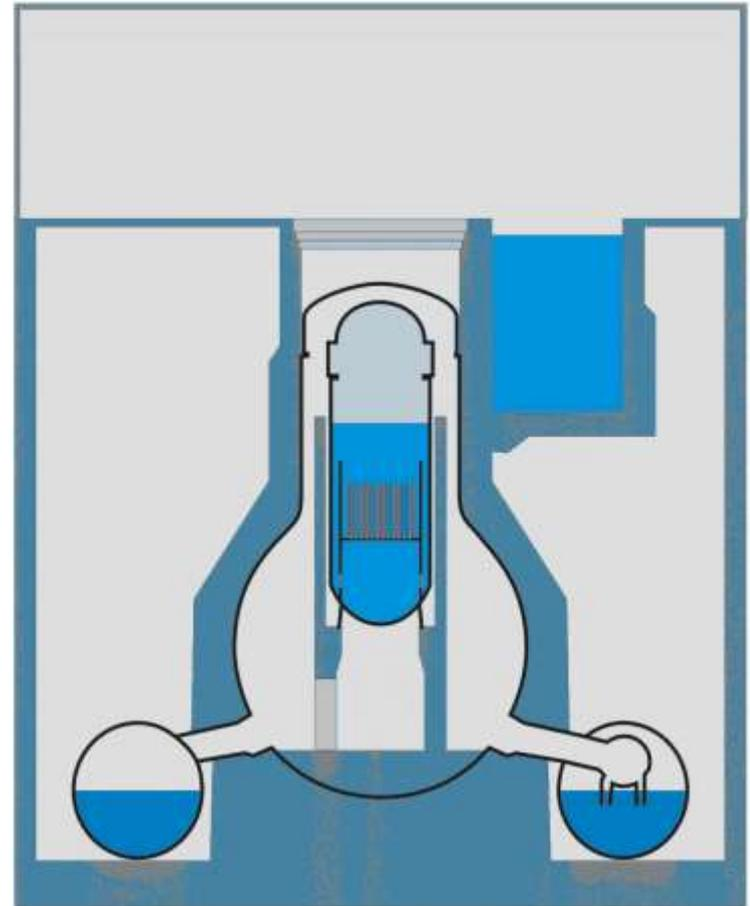
Water begins to be removed from the reactor vessel due to pressure build up
