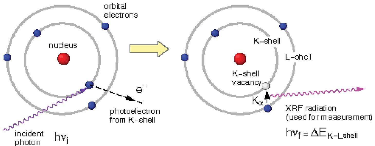
Fig. 1: Generation of XRF radiation by photoelectric effect
