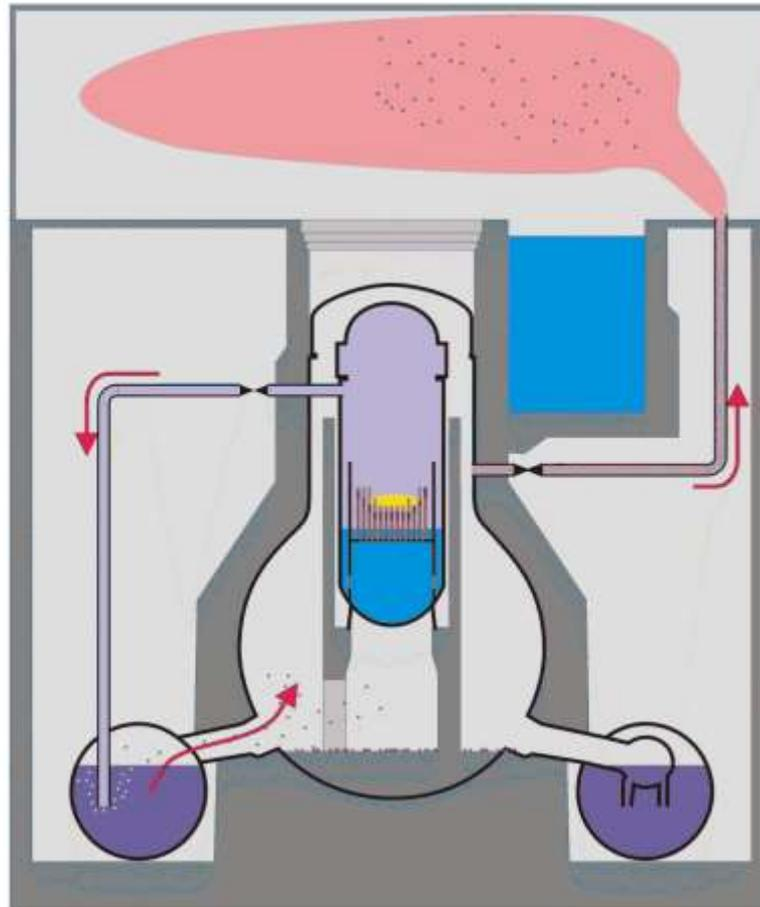
The hydrogen ignites, and no control mechanism for the release of fission products exists. Three out of four of the affected units suffer from a hydrogen explosion. One unit, which had a vent to the outside stuck open, does not explode. Unit 2 has an additional challenge.
