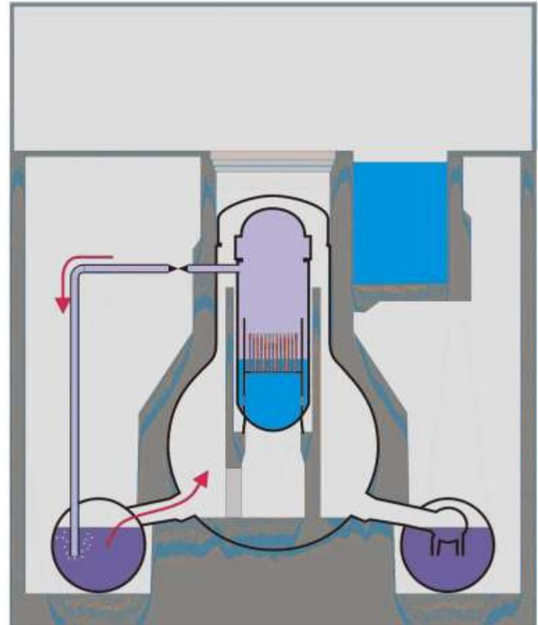
The release of fission products during melt down. This includes the Xenons, Cesium 134, 137, and the radio-Iodines, (~0.1%)
