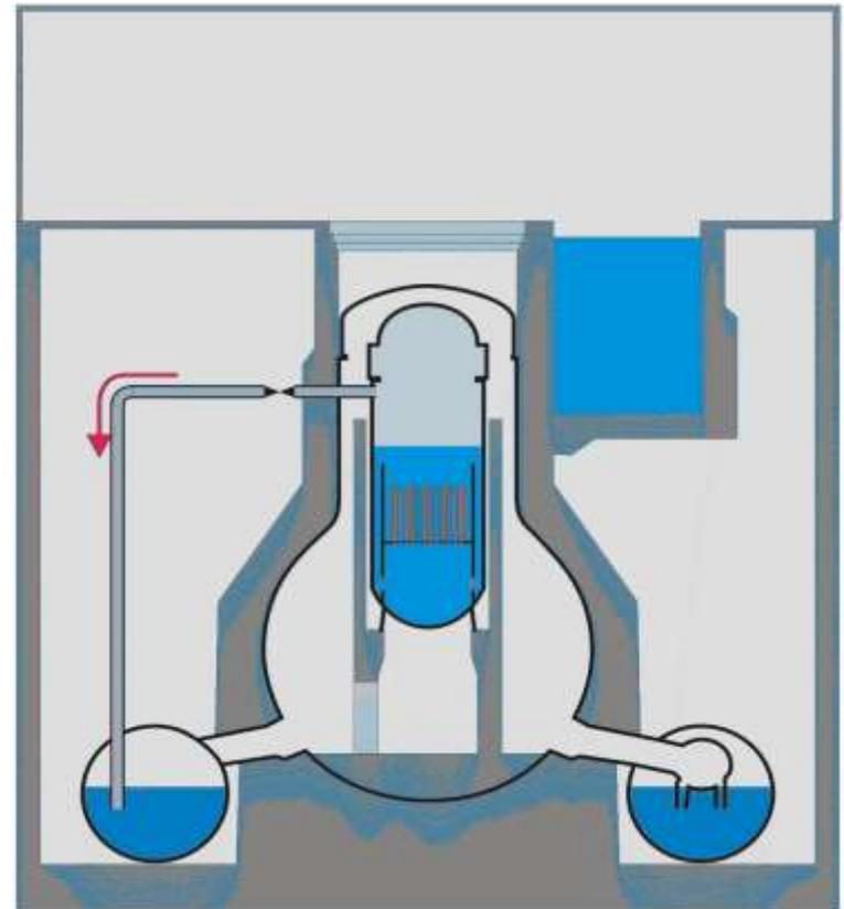
As water is removed, the temperature in the core increases, opening the steam relieve valves discharging steam into the Wet-Well
