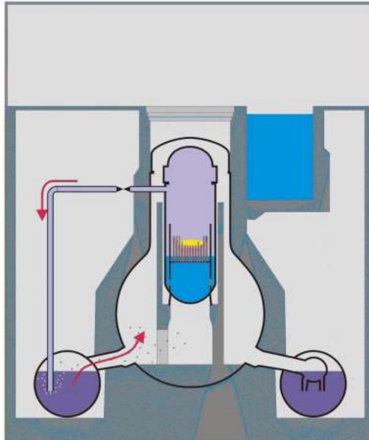
The release of activity begins, and hydrogen build up occurs in the reactor building. Hydrogen is flammable. There are no hydrogen recombining units at the Fukushima BWRs.
