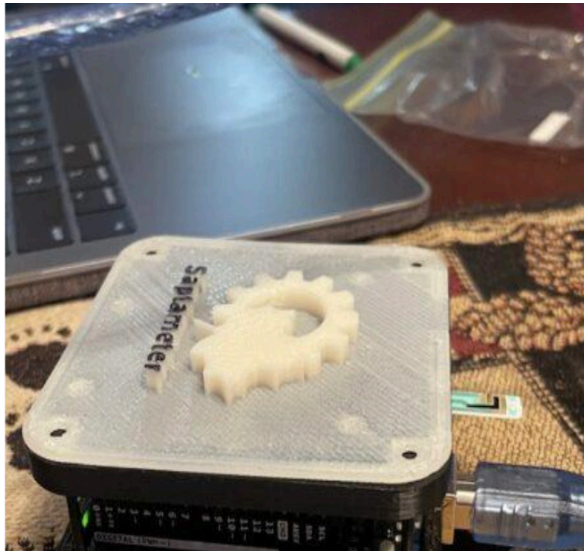
The team developed the Saptameter, a cost-effective, hand-held biosensor that can detect invert sugar levels in maple syrup. It includes a printed circuit board modified to detect different molecules in syrup. (University of Rochester photo / Rochester iGEM team)
