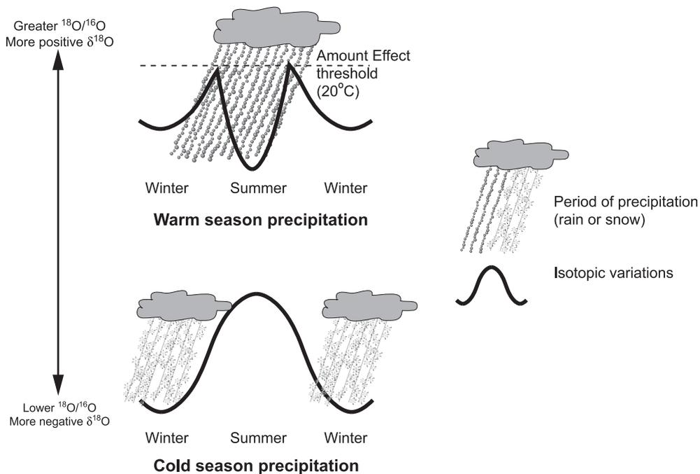
Fig. 1. Illustration of the isotopic effect of heaviest precipitation (rain or snow) during different parts of the year, and the relationship to ambient temperature. Summer rains, when ambient temperatures are greater than about  $20^\circ\text{C}$  result in a marked decrease in the  $^{18}\text{O}/^{16}\text{O}$  ratio in meteoric water (and thus  $\delta^{18}\text{O}$  values).
