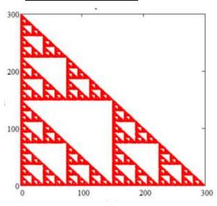
Often, hollow structures have mechanical stability superior to solid material, at lower weight and material cost. Consider the planar structured shape in the figure, which is plotted to scale (300u **X** 300u). The intricate hole structure is self-similar (fractal) on decreasing length scales.
