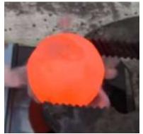
4m x 3.5m. It is exposed to the ambient air (18<sup>o</sup>C), cooling down from its original temperature of T = 1273K by radiating heat energy Q according to the Stefan-Boltzmann Law (assume emissivity  $\varepsilon = 1$ , neglect the effect of the ambient temperature).
