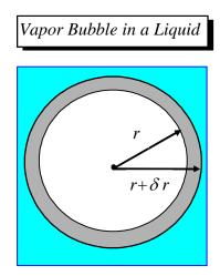
the surface and, hence, the radius of the bubble, and increases the effective pressure inside the bubble. This effect of the surface tension is counteracted by the gas pressure inside the bubble, preventing the bubble from collapsing. *Equilibrium* is achieved, when the *work done by the pressure* for an infinitesimally small change in radius,  $\delta r$ , cancels the change in surface energy:
