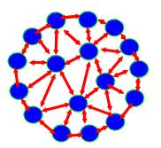
Another type of mechanical energy that is important for liquid and gaseous systems is that of **surface energy** or **surface tension**. As illustrated in the figure, the particles in the interior of a **droplet of matter** are attracted to all sides from their nearest neighbors, such that the resultant force is approximately zero. The resultant force acting on particles in the surface is directed inside (radially inwards). The **pressure**
